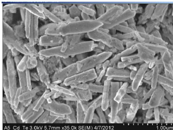
**Figure 4.** SEM images of CdTe nanorods obtained from Cadmium (II) complex of bis-(isopropyltelluro) propane.
