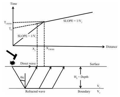
Figure 1. A schematic diagram of compressional wave and travel time curves (After: [9]).
