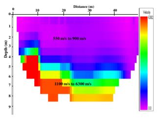
Figure 2. The synthetic velocity model for the test site.
