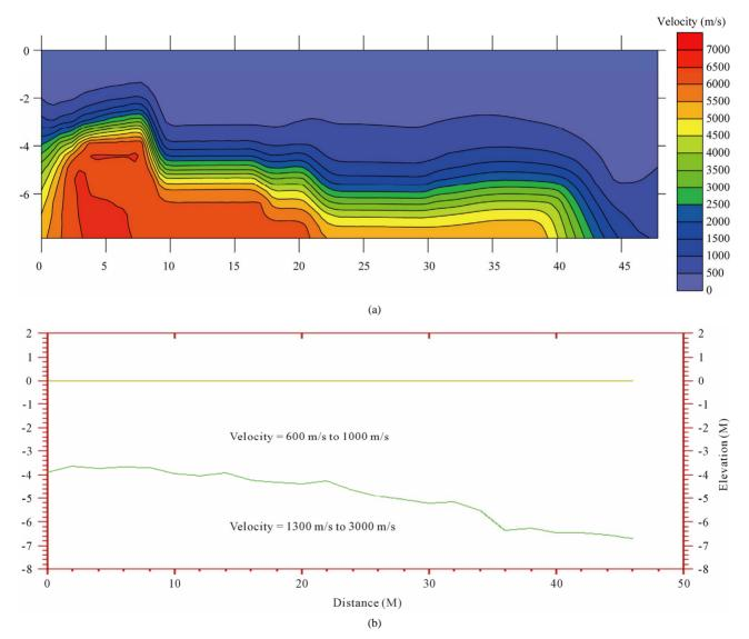
Figure 4. The comparison between the SeisOpt (a) and GREMIX15 (b) velocity model result.
