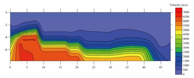
Figure 3. The velocity tomography model for the test site.
