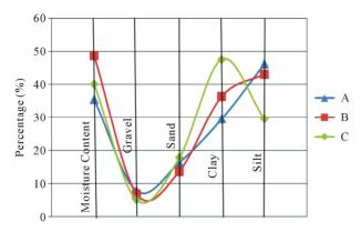
Figure 5. The variation of moisture content, gravel, sand, clay and silt values in percentage for all three tested soil specimen.
