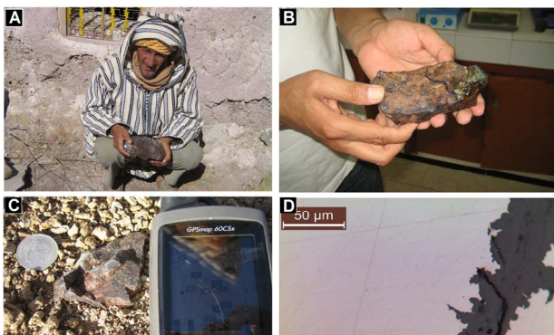
Figure 3. Meteorite fragments of Imilchil. A: Sample of more than 9 kg; B: Sample of more than 1.5 kg; C: Sample of 290 grams on site; D: Band of kamacite in a plessite matrix.
