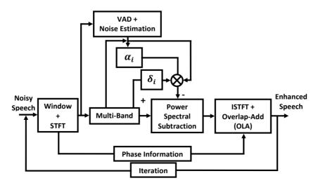
Figure 3. Block diagram of multi-band spectral subtraction exploiting iterative processing algorithm.
