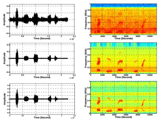
Figure 7. Temporal waveforms and speech spectrogram with sp1 utterance, "The birch canoe slid on the smooth planks", by a male speaker from the NOIZEUS speech corpus: (from top to bottom) noisy speech (degraded by car noise at 5 dB SNR); speech enhanced by MBSS (PESQ = 1.776), and speech enhanced by IP-MBSS (1.915).
