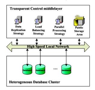
Figure 2. database cluster system framework.
