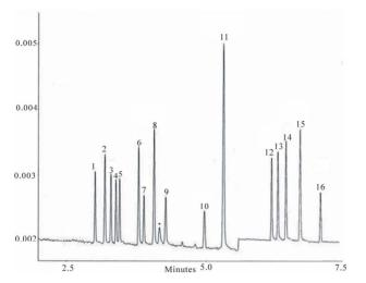
Figure 2. Electropherogram of standard mixture. Peak identification: as in Figure 1. Experimental conditions: Borate buffer 60 mM, pH = 9.2, V = 25 kV (I = 80  $\mu$ A); V = 30 kV (I = 100  $\mu$ A) at t = 5.80 min; p = 20 psi at t = 7.2 min; T = 25°C; injection: 0.5 psi for 5 s; capillary and instrument: as in Figure 1.
