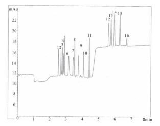
Figure 4. Electropherogram of standard mixture. Peak identification and experimental conditions as in Figure 2 except V = 30 kV at t = 4.6 min and pressurization of inlet vial at t = 6.6 min; fused silica capillary I.D. 50 µm. Instrument Agilent 7100.
