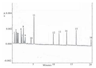
Figure 1. Electropherogram of standard mixture. Peak identification: (1) II, (2) E, (3) CPM, (4) DPH, (5) PM, (6) PE, (7) T, (8) L, (•) EOF, (9) DHE, (10) A, (11) CH, (12) BuP, (13) PrP, (14) EtP, (15) MeP, (16) *p*-HBA. Experimental conditions: Borate buffer 60 mM pH = 9.2; V = 25 kV (I = 80  $\mu$ A); T = 25°C; injection: 0.5 psi for 5 s; fused silica capillary I.D. = 50  $\mu$ m, L = 59.5 cm, I = 49.5 cm; instrument P/ACE MDQ System (Beckman).
