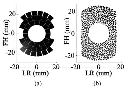
**Figure 1. Schematic for the simulated arrays: (a) concentric ring and (b) random. FH: foot head; LR: left right direction for treatment.**
