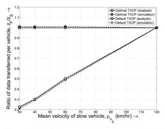
Figure 4. Ratio of data transferred per node vs velocity of slow vehicle with default scheme and TXOP tuning ( $\mu_{v_F}$  = 120 km/hr,  $\sigma_{v_S} = \sigma_{v_F} = 5$  km/hr).
