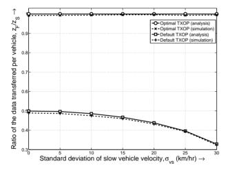
Figure 7. Ratio of data transferred per node vs standard deviation of slow vehicle speed ( $\mu_{vS} = 60$  km/hr,  $\mu_{v_F} = 120$  km/hr,  $\sigma_{v_F} = 5$  km/hr).
