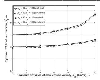
Figure 5. TXOP of fast vehicle vs standard deviation of slow vehicle speed ( $\sigma_{v_F} = 5$  km/hr).
