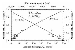
Figure 6. Illustration of  $Q_A$ -SSL<sub>A</sub> and A-SSL<sub>A</sub> relationship.
