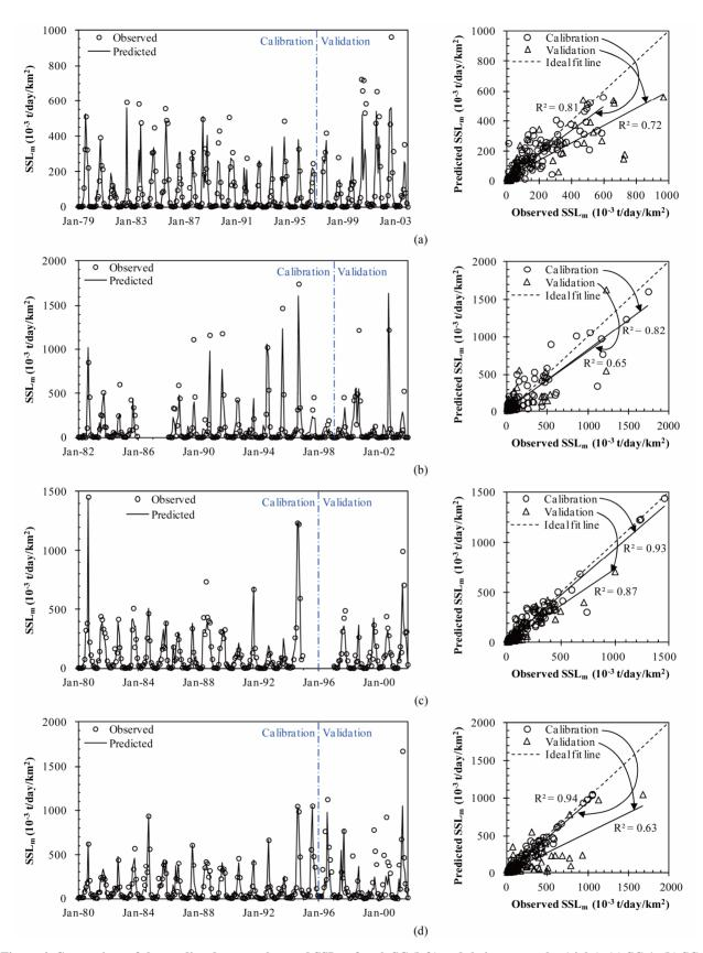
Figure 4. Comparison of the predicted versus observed  $SSL_m$  of each SC (left) and their scatter plot (right). (a) SC-1; (b) SC-2 (no data in 1986 and 1987); (c) SC-3 (no data in 1995 and 1996); and (d) SC-4.
