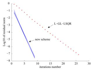
Figure 2. Comparing the new scheme with the  $\mathcal{L}$ -GL-LSQR algorithm with n = 4000 s = 4.
