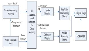
Figure 2. Compound chaos image encryption systemwith time-varying parameters
