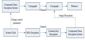
Figure 1. Chaos image encryption/ decryption principle with time-varying parameters
