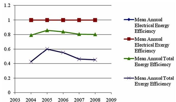
Figure 7. Mean annual efficiencies with zero generator diesel.
