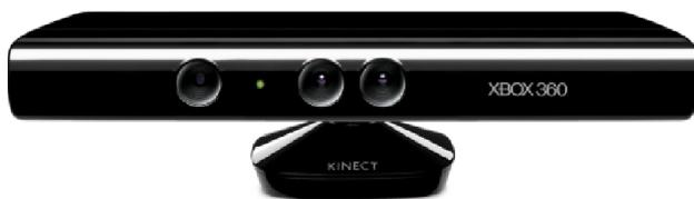
**Figure 1.** The Kinect device with (from left to right) laser projector, RGB camera, and NIR camera.
