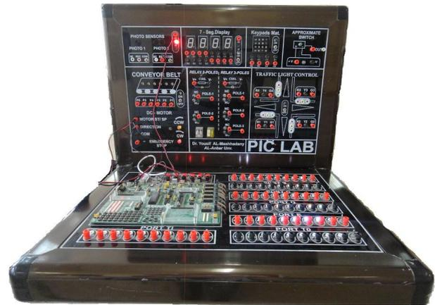
**Figure 3.** The PIC-microcontroller-based conventional electronic control trainer.
