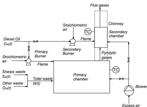
Figure 1. Design features of the assessed incinerator.
