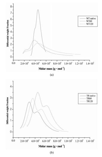
Figure 2. (a) Plot of Differential Weight Fraction vs Molar Mass for enzyme WT proteins prior to (WT native), and after illumination with WLPL for 60min (WT60) and 120 min (WT120); (b) Plot of Differential Weight Fraction vs Molar Mass for enzyme TR proteins prior to (TR native) and after illumination with WLPL for 60 min (TR60) and 120 min (TR 120).
