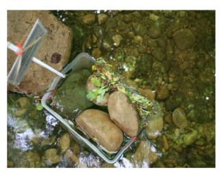
Figure 1. Experimental setup: Exposure of a basket with 5 plexiglass cages in the Hornbach at the downstream site. Photo A. Gerhardt.
