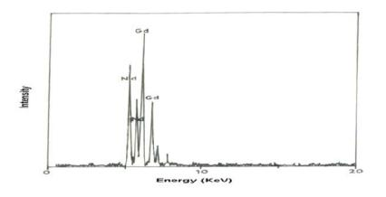
Figure 2. EDAX spectrum of GNO crystals
