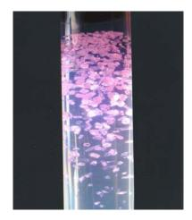
Figure 1. Growth system of GNO crystals
