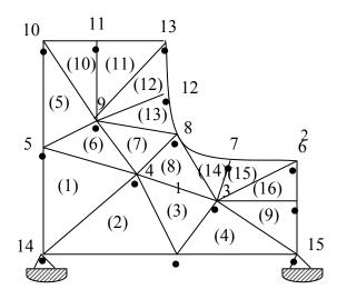
Figure 1: Idealized Finite element Model of two Dimensional Composite Body.
