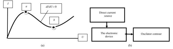
Figure 4. The oscillator with negative active conductivity: (a) Volt-ampernaja the characteristic; (b) The block diagram.
