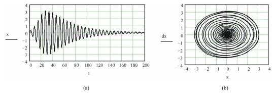
Figure 6. Transient (a) and a phase portrait (b) the oscillator with compulsory attenuation.
