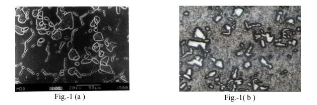
Figure 1. (a) & (b) Show microphotographs of Al-Ti Master alloys prepared at  $800^{\circ}$ C-45min and  $900^{\circ}$ C-45min respectively
