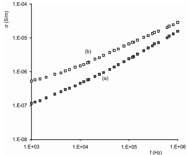
**Figure 4.** A typical set of experimental datasets demonstrating the behaviour of the ac conductivity with respect to frequency for both (solid squares, a) type-1 and (open squares, b) type-2 specimens.
