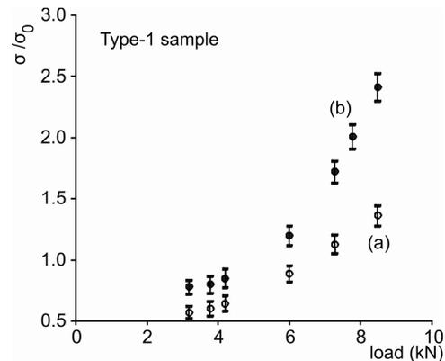
**Figure 8.** Representative plot of the behaviour of ac conductivity for all type-1 specimens in both before (b) and after (a) removing their natural moisture.
