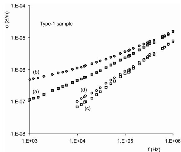
**Figure 7.** Representative experimental datasets of the ac conductivity in the frequency range between 1 k Hz - 1 MHz for type-1 specimen. (a) and (b) correspond to the specimens that maintained their natural moisture before and after applying mechanical load (7.3 kN) respectively. (c) and (d) correspond to the specimens after removing their natural moisture before and after applying mechanical load respectively.
