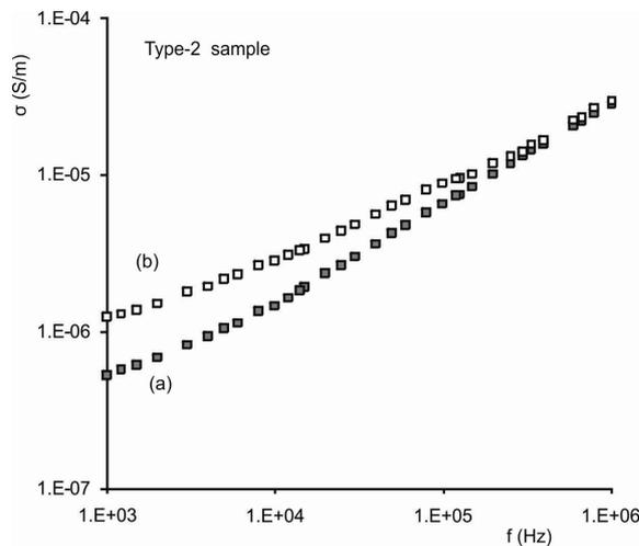
**Figure 6.** A typical set of experimental datasets demonstrating the behaviour of the ac conductivity with respect to frequency for type-2 specimen (solid squares, a) before and (open squares, b) after applying 8.5 kN mechanical load.
