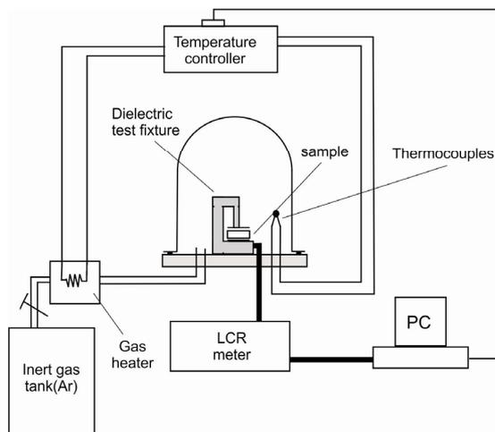
**Figure 3.** Dielectric measurements arrangement including the inert gas tank.
