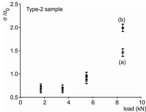
**Figure 9.** Representative plot of the behaviour of ac conductivity for all type-2 specimens in both before (b) and after (a) removing their natural moisture.
