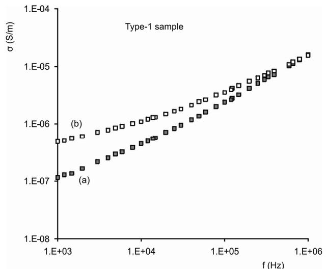
**Figure 5.** A typical set of experimental datasets demonstrating the behaviour of the ac conductivity with respect to frequency for type-1 specimen (solid squares, a) before and (open squares, b) after applying 7.3 kN mechanical load.
