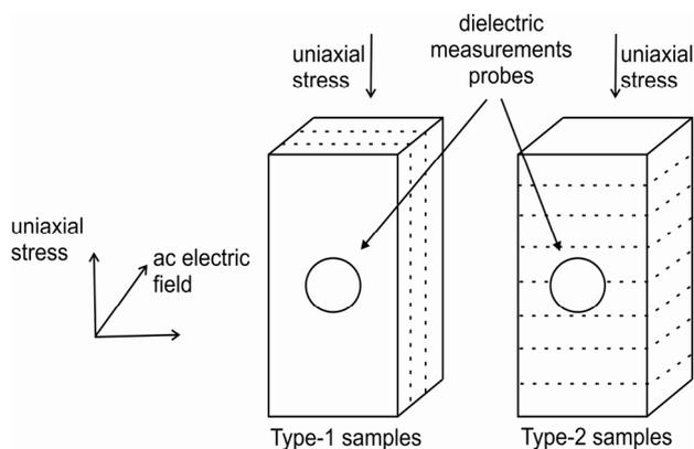
**Figure 1.** Orientation of the specimens according to the directions of the applied stress, the dielectric measurement probes and the conductive layers of muscovite and chlorite (type-1 and type-2 specimens).
