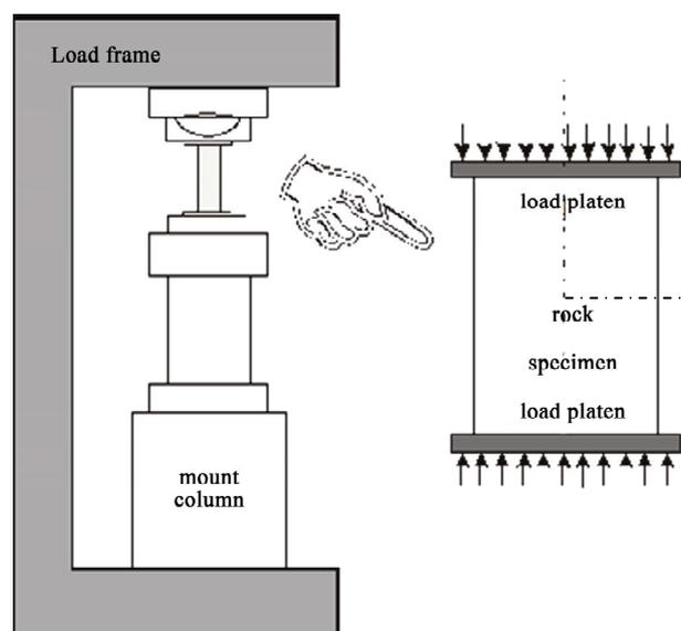
**Figure 2.** Typical testing system for uniaxial compression testing.
