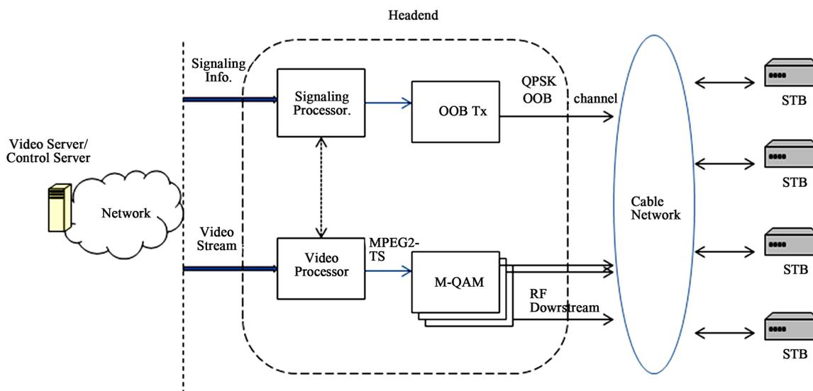
**Figure 3. OOB-based cable network.**
