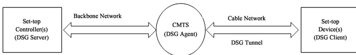
**Figure 2. Logical diagram of DSG system.**
