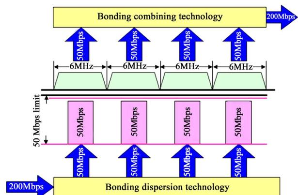
**Figure 1. Example of channel bonding.**
