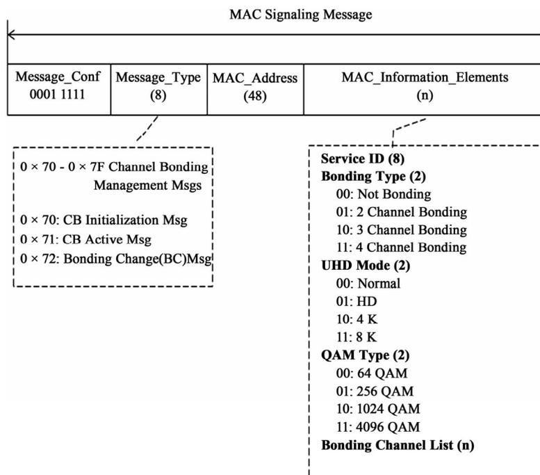
**Figure 5. Signaling message of OOB-based protocol.**
