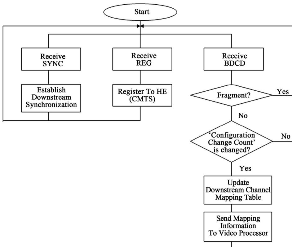
**Figure 10. Procedure of the BDCD message at a STB.**
