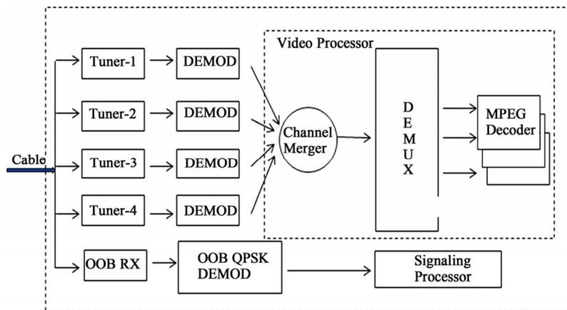
**Figure 4. Function Block Diagram of the STB in the OOB-based cable network.**
