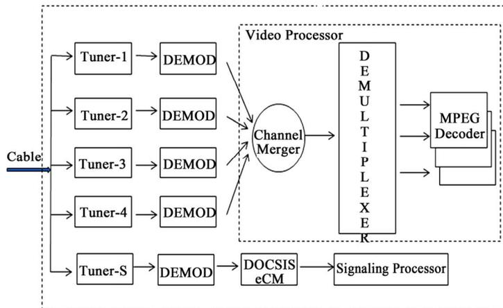
**Figure 8.** Function block diagram of the stb in the DSG-based cable network.
