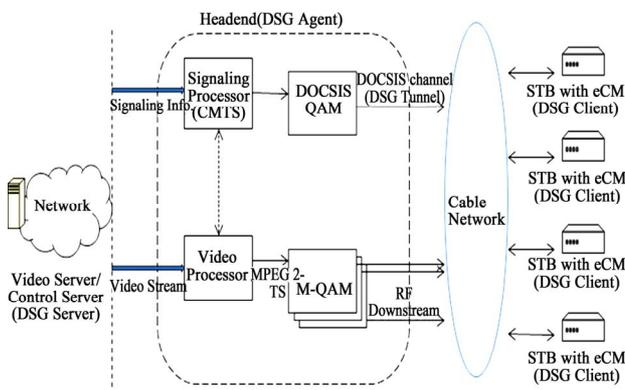
**Figure 7. DSG-base cable network.**
