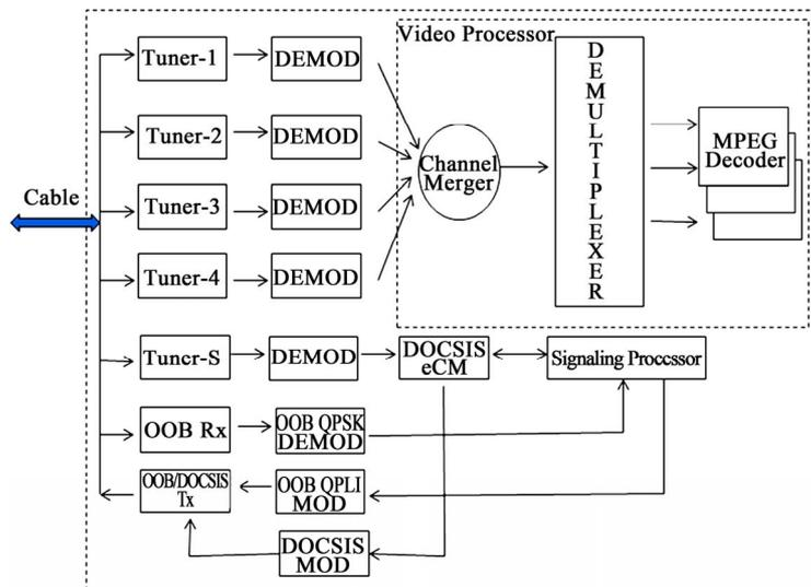
**Figure 9.** Function block diagram of the STB for two-way transport.
