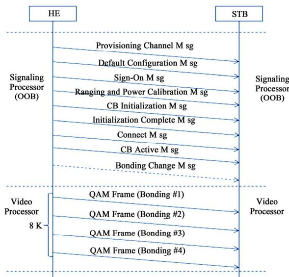
**Figure 6. Message flow in OOB-based cable network.**
