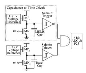
Figure 4. Capacitance-to-time circuit.
