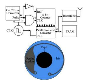
Figure 5. Device block diagram and frontal view of implantation.
