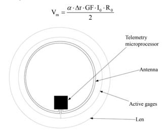
Figure 3. Contact lens wireless sensor.
