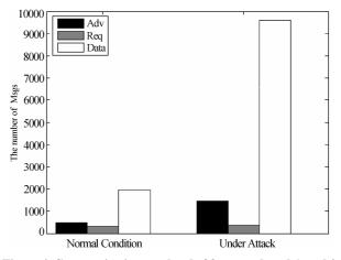
Figure 4. Communication overhead of free attack and Attack2.
