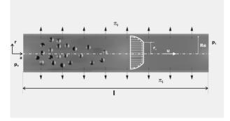
**Figure 1.** Longitudinal transport of molecules or nanoparticles in a blood capillary with a blunted velocity profile.
