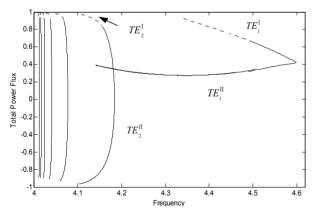
Figure 5. The total power flux of the higher-order *TE* guided modes. The curves are arranged along horizon-tal-axis with m = 7, 6, 5, 4, 3, 2, 1, respectively. The dashed curves stand for  $TE_m^1$  modes, the solid curves correspond to  $TE_m^{\Pi}$  modes
