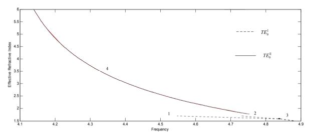
Figure 2. The dispersion curves of the fundamental *TE* guided modes, the effective-refractive-index is a function of frequency. For  $TE_0^{\perp}$  mode, the curves 1, 2, 3 correspond to  $h_1 = 0.1$  cm, 1 cm, 10 cm. For  $TE_0^{\perp}$  mode, only one curve 4 for  $h_1 = 0.1$  cm, 1 cm, 10 cm
