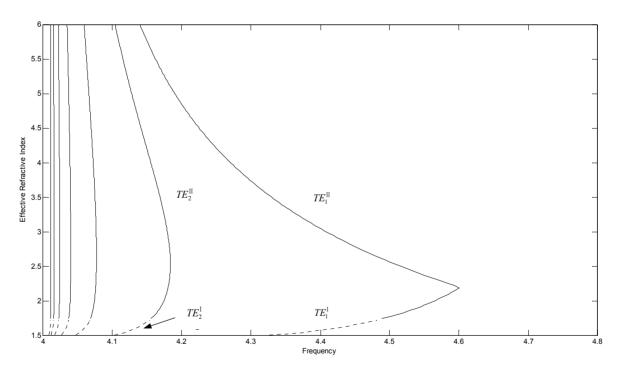
Figure 3. Dispersion curves for higher order *TE* guided modes, the effective-refractive-index is a function with frequency. The curves are arranged along horizontal-axis with m = 7, 6, 5, 4, 3, 2, 1, respectively. The dashed curves stand for  $TE_m^1$  modes, and solid curves correspond to  $TE_m^{11}$  modes
