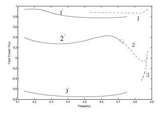
Figure 4. The total power flux of the fundamental *TE* mode for different slab thicknesses. The parameters are the same as Figure 2. The dashed curves stand for  $TE_0^{I}$  modes, the solid curves correspond to  $TE_0^{II}$  modes
