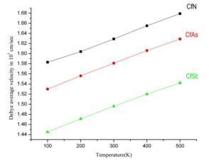
Figure 3. Debye average velocity versus temperature along <111> direction.
