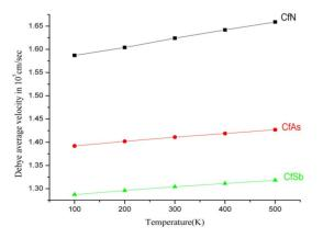
Figure 2. Debye velocity versus temperature along <110> direction.
