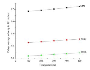
Figure 1. Debye average velocity versus temperature along <100> direction.
