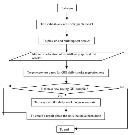
Figure 1. Developing flow of GUI automation test system
