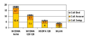
Figure 14. VoIP call signaling delays.
