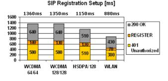
Figure 13. SIP registration signaling delays.
