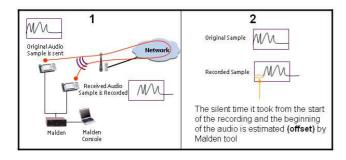
Figure 11. Offset delay measurement environment.
