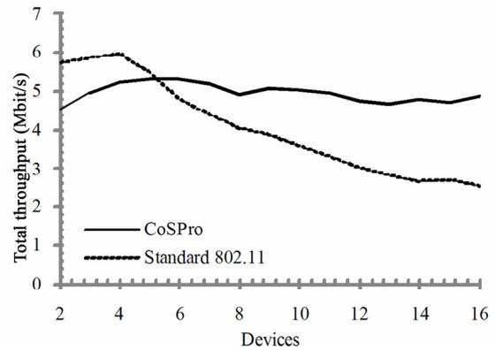
Figure 12. Measured network throughput with and without CoSPro.
