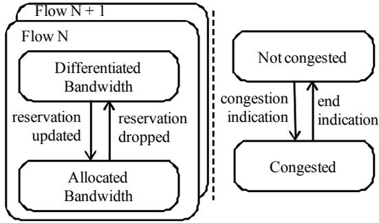
Figure 5. QoS states in a CoSPro end device.
