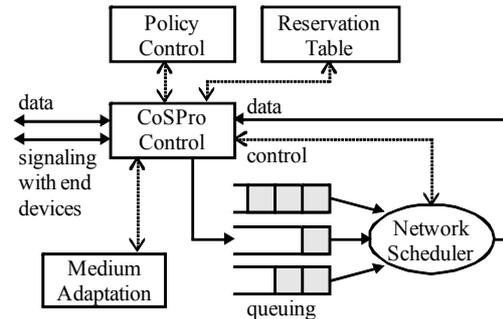
Figure 4. Functional architecture of the CoSPro controller.
