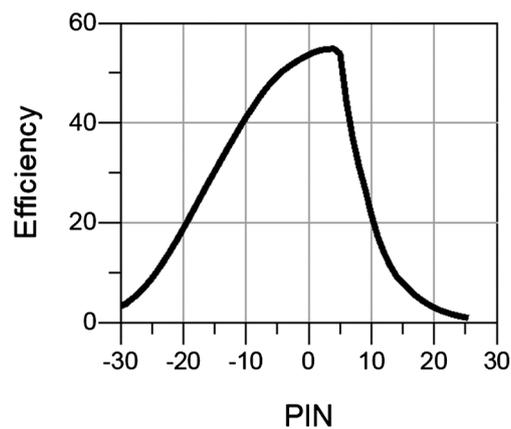
Figure 8. Single band rectifier: RF-to-dc conversion efficiency versus input power (dBm).
