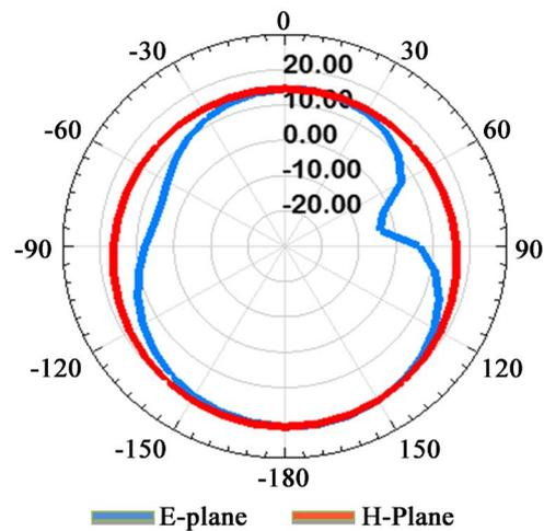
Figure 5. Radiation patterns of the antenna at 2.45 GHz.
