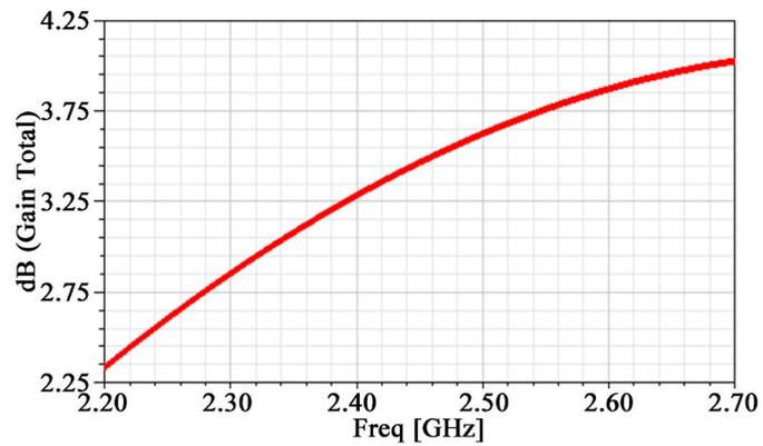
Figure 4. The antenna gain at 2.45 GHz.
