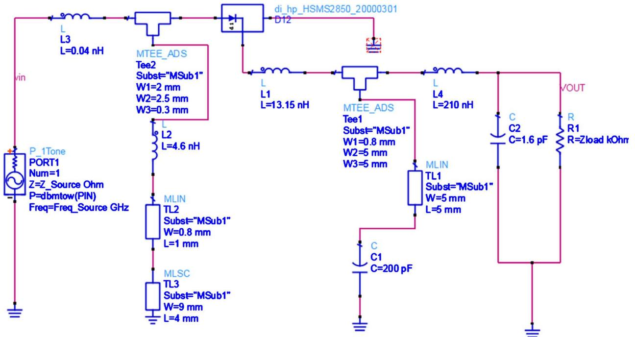
Figure 6. Simulation of the adaptation and rectification circuit.
