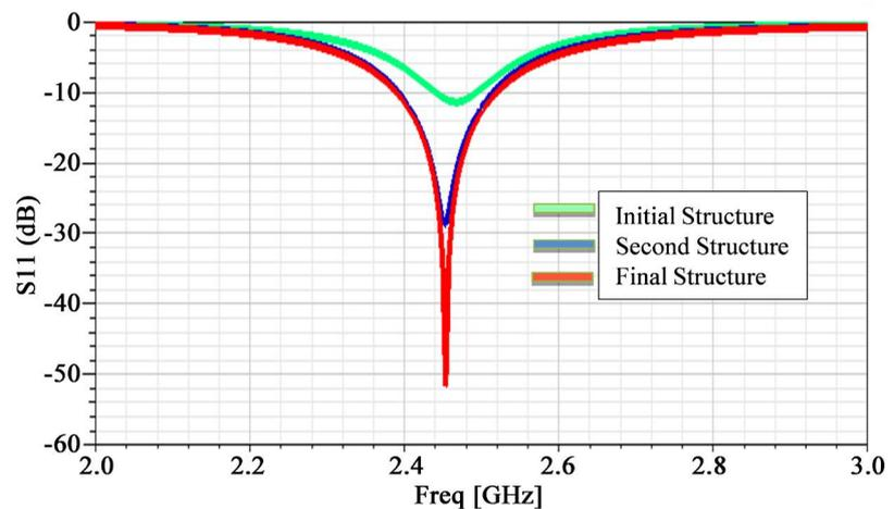
**Figure 3.** Reflection coefficient variation from initial to final structure.**Table 2.** Results of the reflection coefficient (S11) and gain as a function of frequencies.
