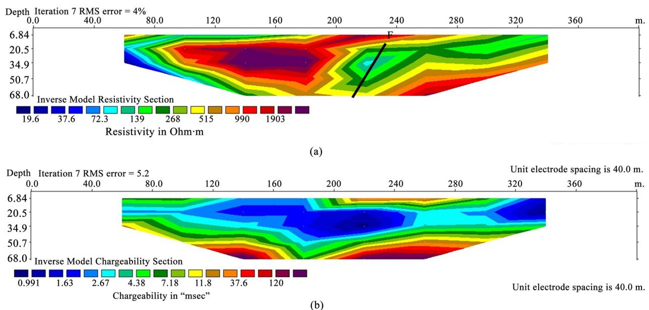
**Figure 5.** Dipole-dipole sections of resistivity and chargeability of dipole spacing of 40 m along Line 596,240 of Um Salim area, central eastern desert, Egypt.
