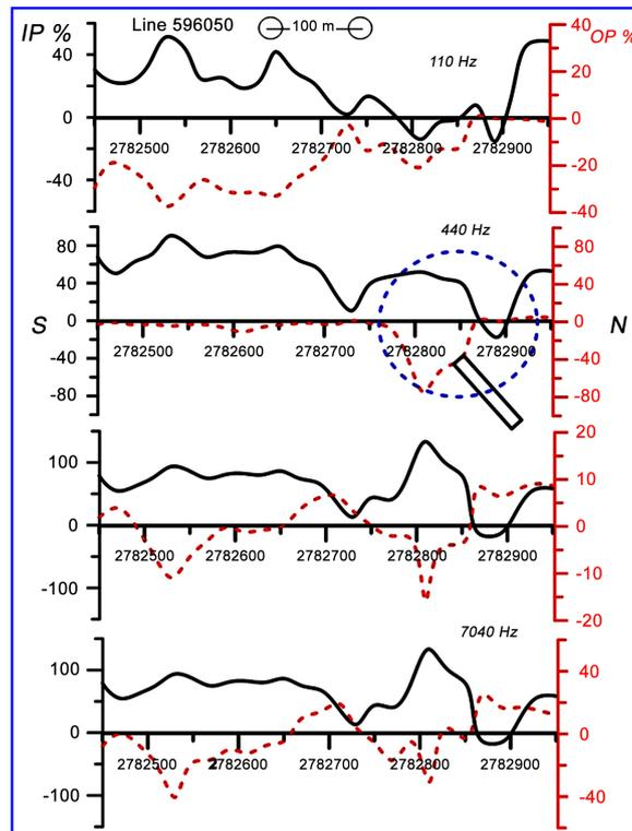
**Figure 3.** Horizontal loop electromagnetic profile line (596,050) of Um Salim area, central eastern desert, Egypt.
