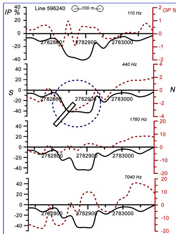
**Figure 4.** Horizontal loop electromagnetic profile line (596,240) of Um Salim area, central eastern desert, Egypt.
