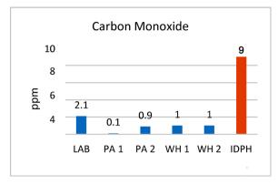
Figure 12. Indoor carbon monoxide data.
