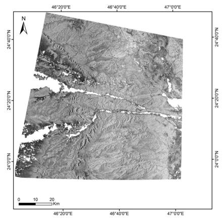
**Figure 10.** Amplitude differential interferometry SAR results of the 26/05/2004 and 31/01/2005 pair from the southern region of Riyadh (resolution 20 m).
