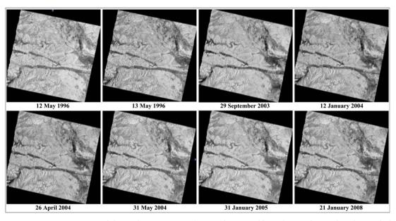
Figure 3. Intensity images of the study area at a resolution of 20 m, calibrated, georeferenced, orthorectified and filtered.
