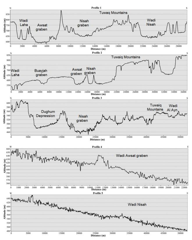
**Figure 7.** DEM topographic profiles of the intensity image; locations of these profiles are outlined in **Figure 6**. Profile 1: across the Tuwaiq Mountain, cutting Wadi Laha, Nisah and Awsat grabens, from north to south. Profile 2 across the Tuwaiq Mountain, cutting Wadi Laha, Nisah and Awsat grabens, from north to south. Profile 3: across the Dughum depression and Nisah Graben. Profile 4: along Al Awsat Graben from west to east. Profile 5: along Nisah Graben from west to east.
