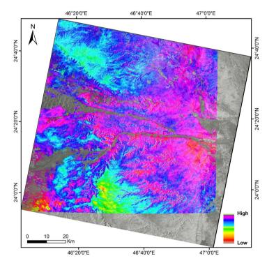
**Figure 9.** The DInSAR interferometry results of the 26/05/2004 and 31/01/2005 pairs for the southern region of Riyadh (resolution 20 m). Altitude values (*x*) are not provided with a numbered scale for unknown coefficient (*k*) value in the following equation:  $x = 2k\pi$ . If *k* for example is equal to 1, the lowest altitude value is equal to  $2\pi$ . Therefore, the interval of the provided range is equal to 50 m/colour, ranging from 400 m to 1000 m according to the topographic map.
