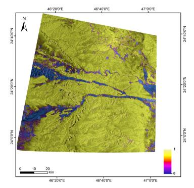
**Figure 8.** The coherence results of the 26/05/2004 and 31/01/2005 pairs for the southern region of Riyadh (resolution 20 m).
