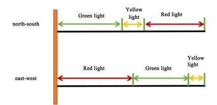
Figure 2. Traffic light system control rules.
