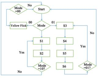
Figure 3. Traffic light system flow chart.
