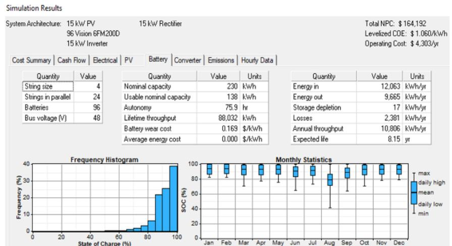
Figure 10. Battery bank state of charge results.
