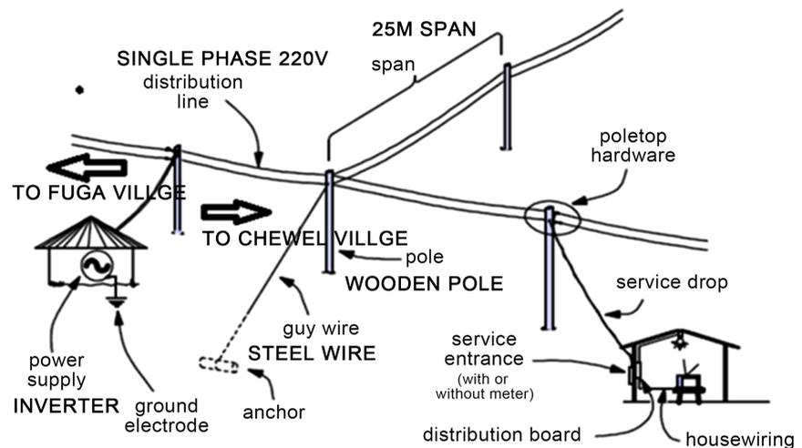
**Figure 4.** Chewel/Fuga mini-grid layout.
