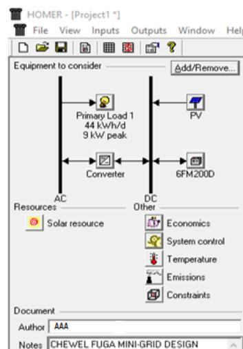
**Figure 6.** HOMER Inputs window, for modelling a 15 kW PV system for Chewel and Fuga villages.
