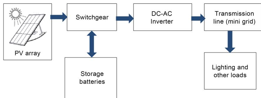
**Figure 3.** Typical PV system components.
