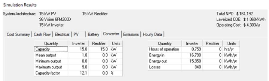
Figure 11. Inverter output results.
