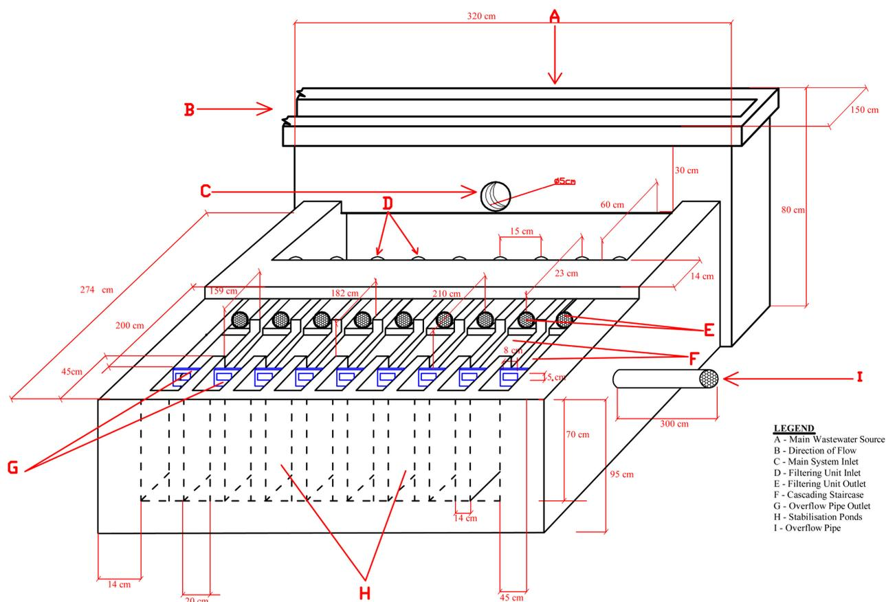
**Figure 4.1: A SCHEMATIC DIAGRAM OF SAND FILTERING UNITS AND FARM STABILIZATION PONDS**
