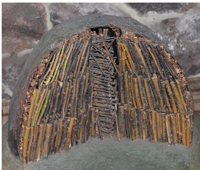
Figure 4. Structure of a charcoal pit, notice the triangular chimney in the middle, the tiers of wood, the leaves covering the wood, and the earthen covering (Photo by Doug Page).
