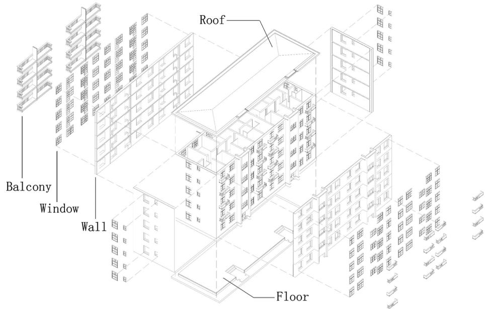
Figure 5. Layer of building-21 envelope system.
