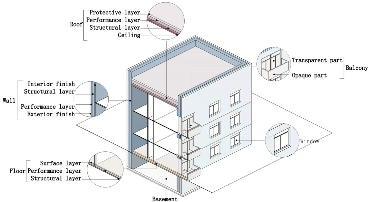
Figure 2. The parts and layers of the existing residential envelope system.
