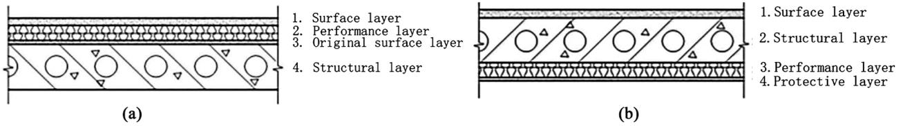
**Figure 4.** (a) Insulation added on the top, (b) Insulation added at the bottom.
