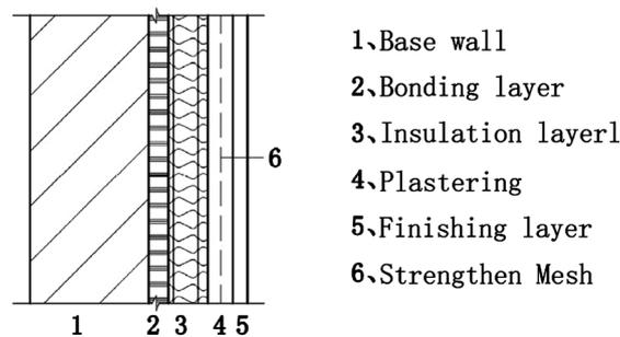
**Figure 3.** External insulation system.
