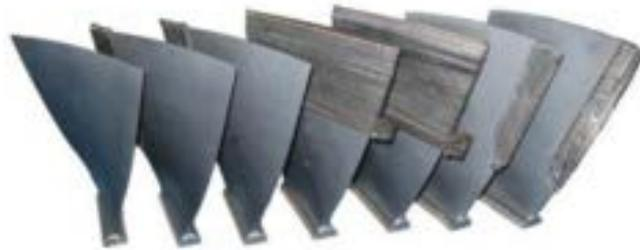
**Figure 6.** The repaired turbines via AM.
