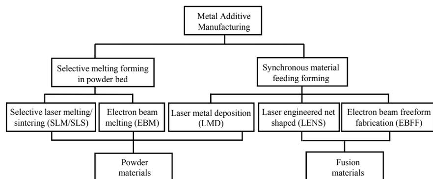
**Figure 1.** Classification of metal additive manufacturing technology.
