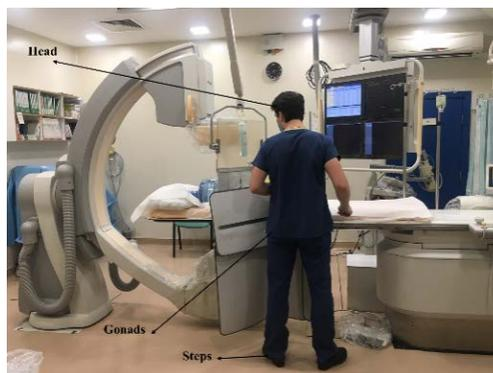
**Figure 4.** Position of cardiologist in relation to patient table, G-arm, radiation protection shield. Measuring points: head, gonads and steps.
