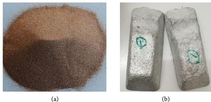
Figure 1. (a) Zircon sand particles (b) ZA-27 ingot.
