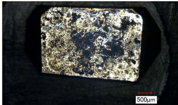
**Figure 6.** Optical microscope image of diamond (110) sample 2 with Bi powder after heating at 540 K (270°C).
