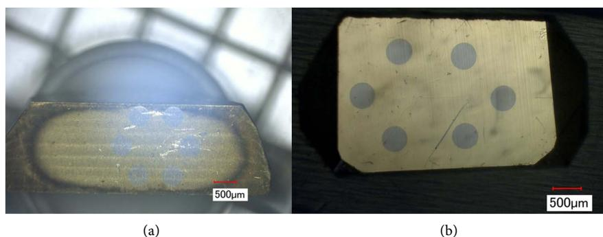
**Figure 2.** Artificial diamond sample images after FIB fabrication, (a) Sample 1 diamond (110); (b) Sample 2 diamond (110).
