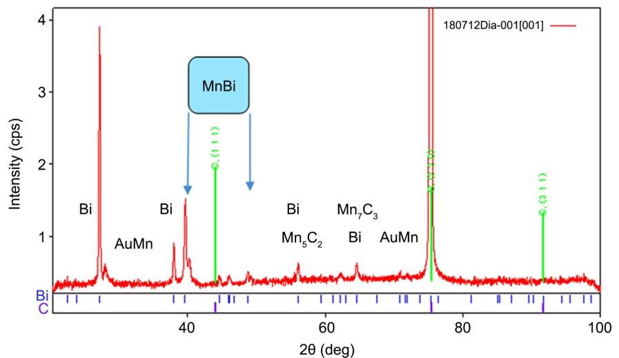
**Figure 7.** X-ray diffraction pattern of the modified diamond (110) with the manganese and bismuth powder.
