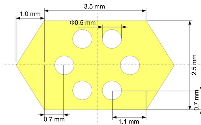
**Figure 1.** Dimensions of the holes of gold covered film on diamond fabricated by focused ion beam.
