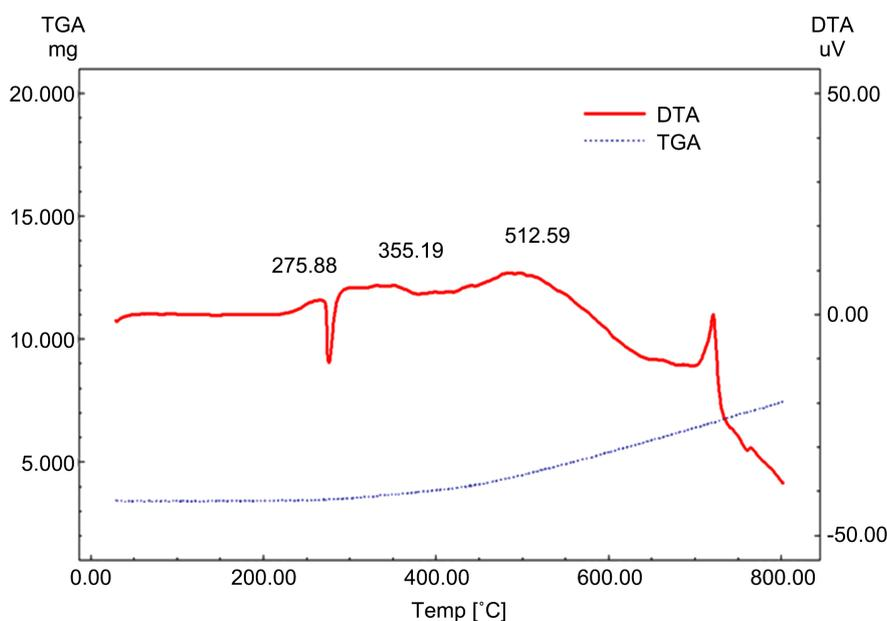
**Figure 4.** Differential thermal analysis curve for diamond powder and manganese powder and bismuth powder.
