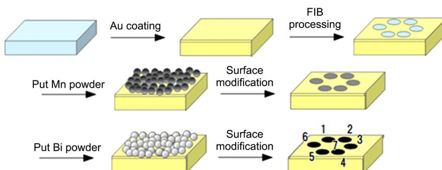
**Figure 3.** Procedures of surface modification using Mn powder and Bi powder on the gold coated surface of diamond.
