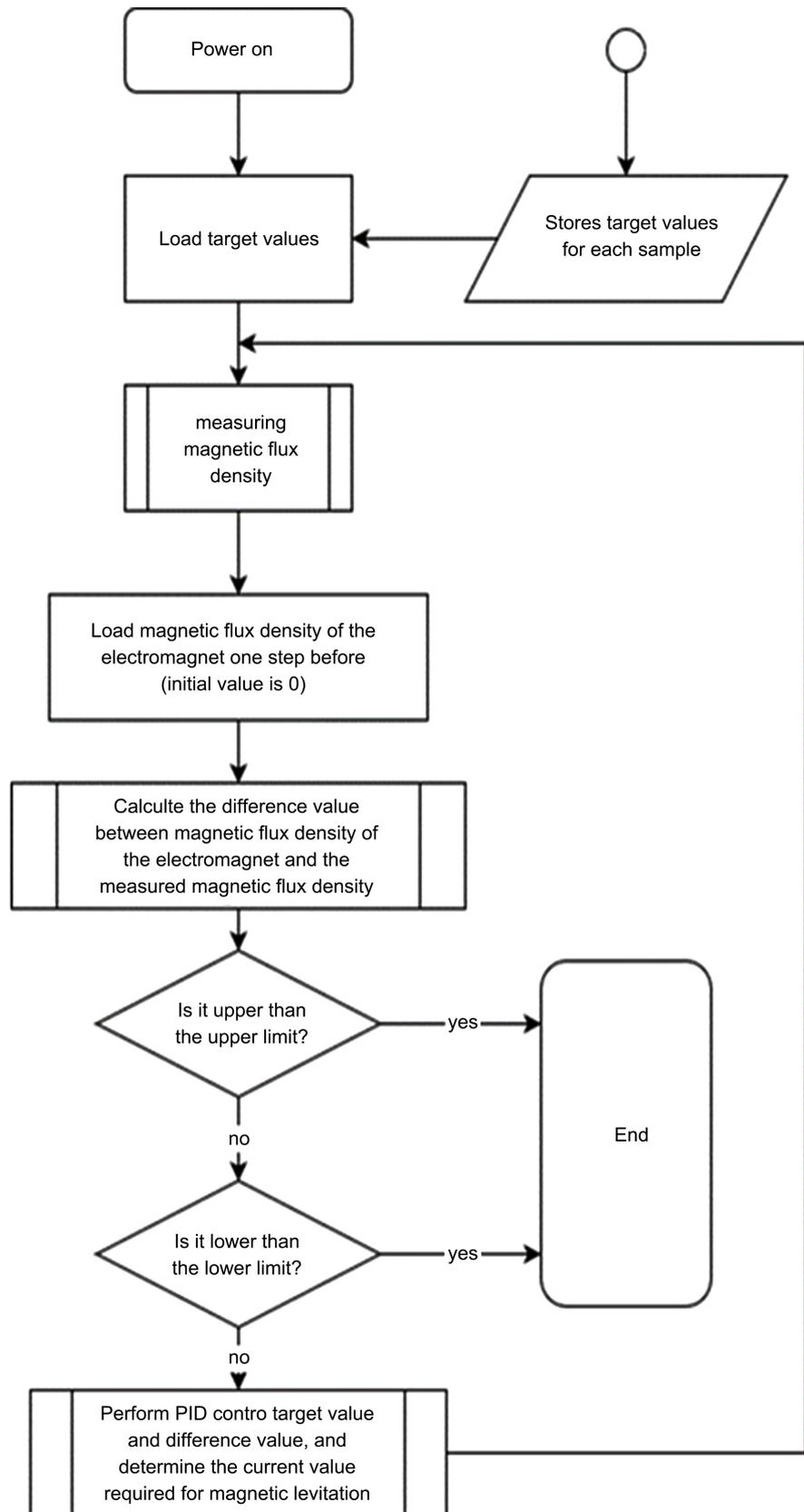
**Figure 9.** Flow chart of the levitation by measuring the magnetic flux by Hall effect sensor attached to upper solenoid coil.
