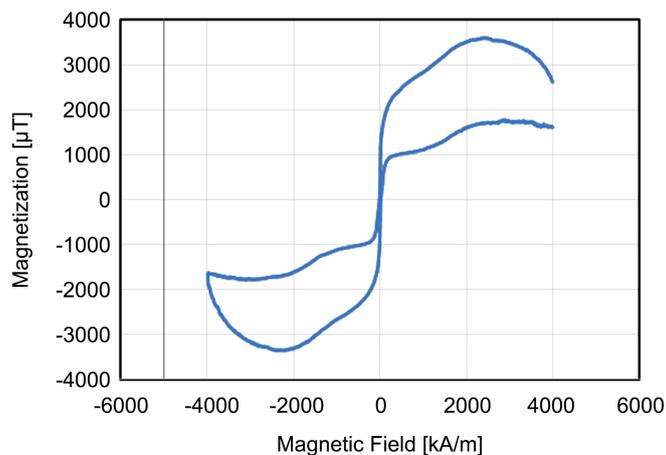
**Figure 8.** M-H curve of sample 2 measured at 10 K.
