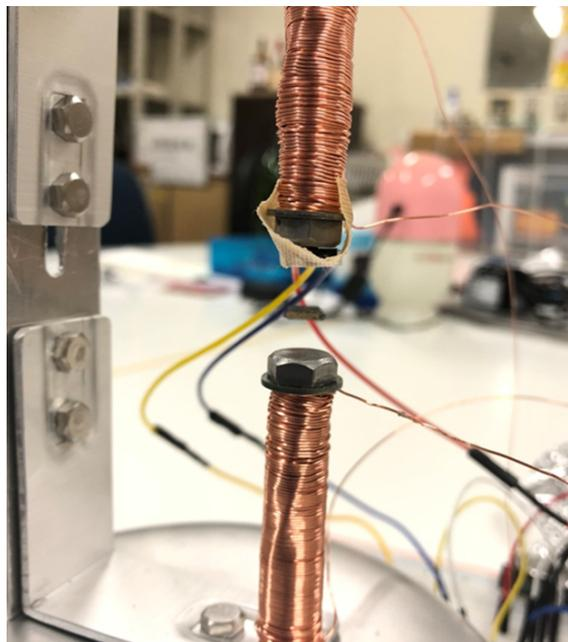
**Figure 10.** Magnetic levitation of the diamond sample 2 using two solenoid coils.
