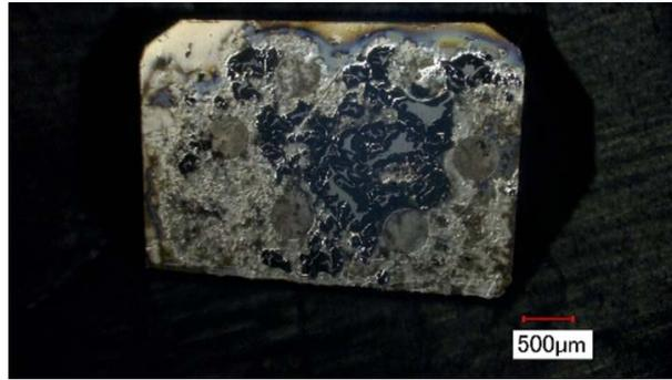
**Figure 5.** Optical microscope image of diamond (110) sample 2 by using manganese powder after the surface modification in the vacuum infrared ray heating furnace.
