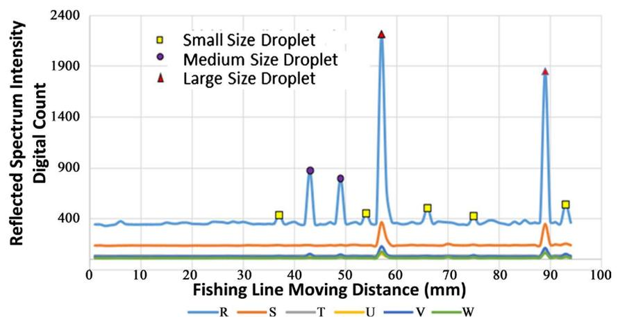
**Figure 4.** Detection of 9 droplets distributed over the fishing line at 6 wavelengths of the NIR sensor.
