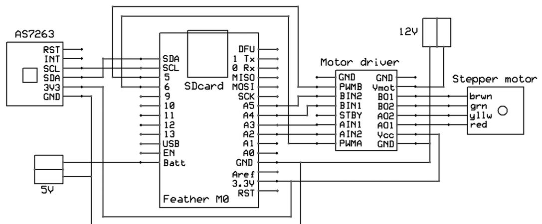
**Figure 2.** Electronic schematic of the system prototype.
