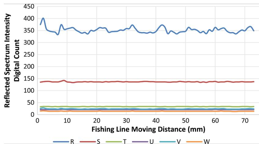
**Figure 3.** Effect of fishing line colors to 6 wavelengths of the NIR sensor.
