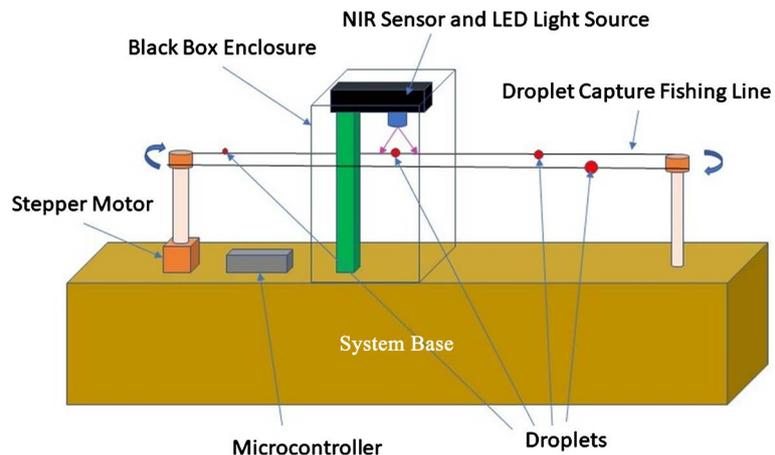
**Figure 1.** Schematic diagram of the optical spray droplet detection system prototype.
