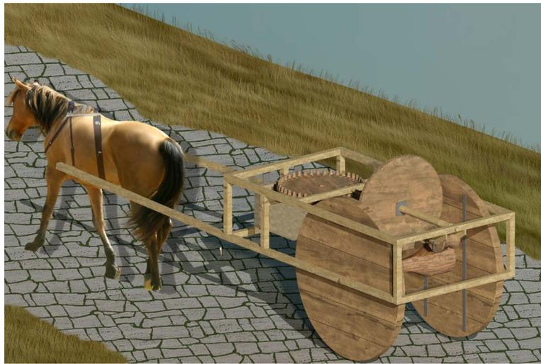
**Figure 7.** Digital reconstruction of Leonardo's odometer.
