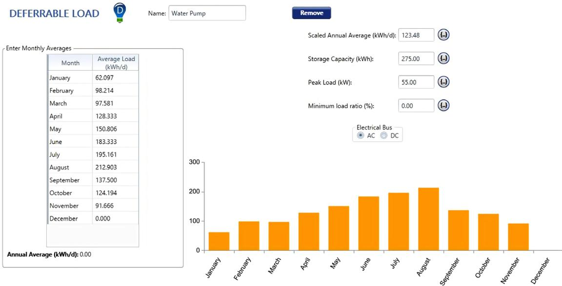
Figure 17. Load mapping in HOMER.
