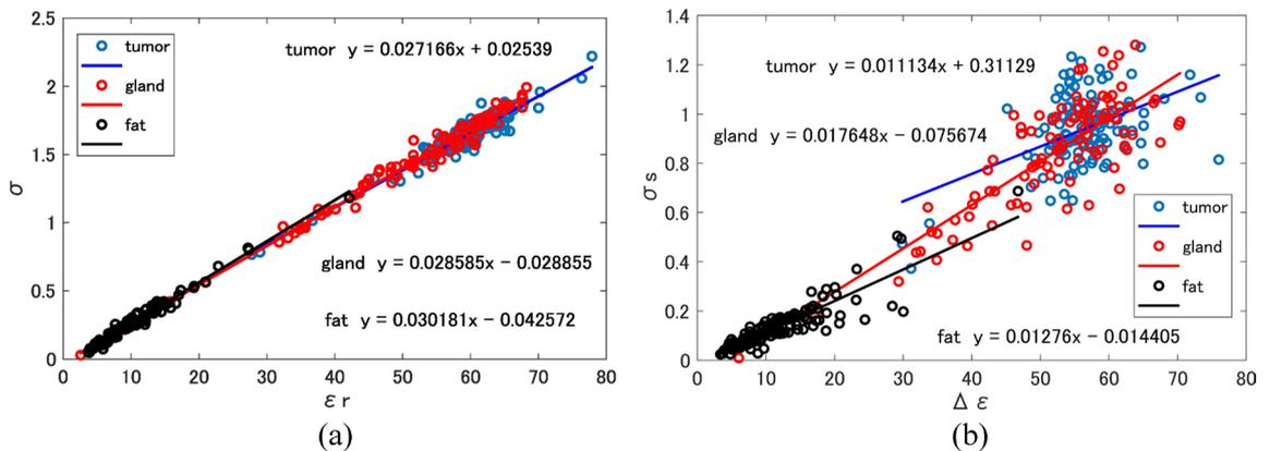
Figure 7. Linear relationship between relative permittivity and conductivity. (a)  $\epsilon_r$  vs.  $\sigma$  (b)  $\Delta \epsilon$  vs.  $\sigma_s$ .
