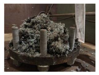
**Figure 19.** Debris obtained from experiment with M/W = 0.41.
