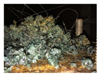
**Figure 11.** Debris obtained from experiment with M/W = 0.11.
