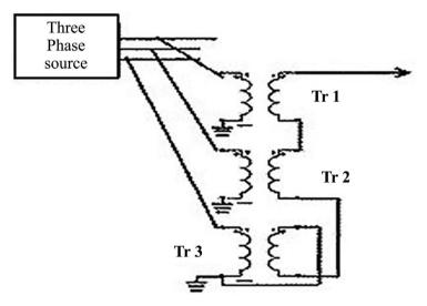
Figure 6. The converter 3 - 1 scheme.
