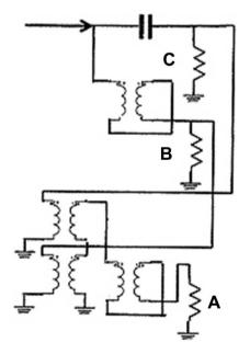
Figure 7. One-way signal converting to three-phase (A, B and C) signals.
