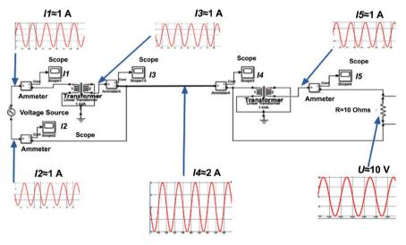
Figure 3. One wire scheme with one phase output.
